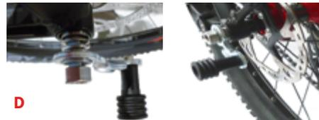
The more centric the alignment of the coupling is, the better the Monoporter coasts.
